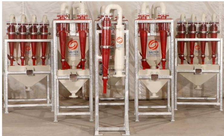
are in-line. Each of the six packages is a stand-alone unit including frame, distributor, valves, piping and launders. Following a successful trial with the pilot plant a full scale system will treat 40 tph.
