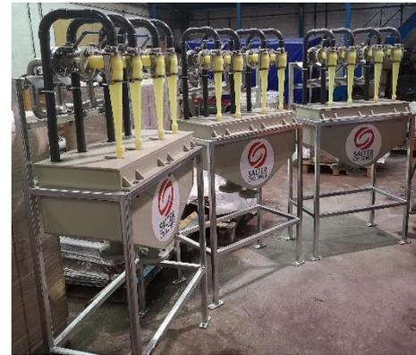
Each Hydrocyclone is fitted with an isolating valve so that individual Hydrocyclones can be taken off-line during planned maintenance periods.
