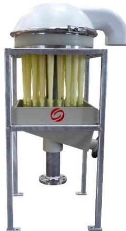
**EXPORTING TO CHINA** A longstanding client operating in China wanted to upgrade the 2" equipment supplied by us in 2012 and we have just despatched a 30 way 2" Mushroom Assembly complete with stand and launders. Each Hydrocyclone vortex finder was fitted with a ceramic extension to further reduce residue in the product.
