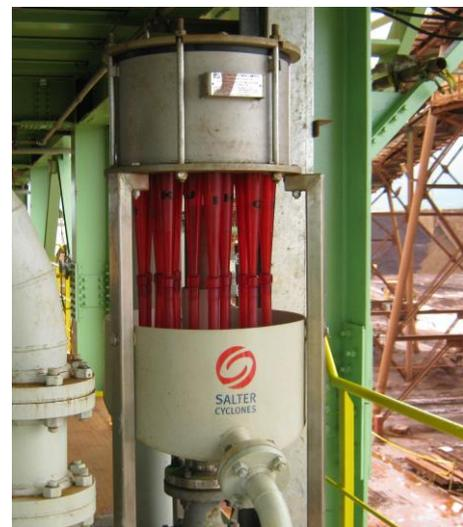
*SC2018 - 18 way 2 inch Canister Assembly operating as a pilot unit on site in Far East*
