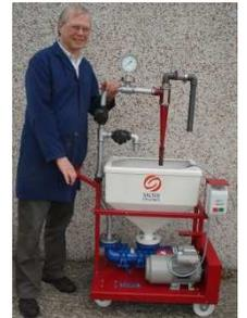
Additionally SCTR1Test Rigs have been supplied to Australia, Singapore, Japan and UK for a wide range of applications including graphene production, slurry recycling and hematite separation.
