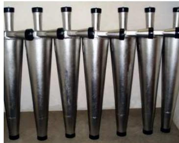
New design stainless steel Germ Clones have been installed to treat a distillery's spent wash reject slurry in order to recover valuable components for return to the revenue stream.
