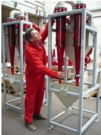
for a dust treatment system and salt washing. Two 2-way five-inch Hydrocyclone packages were supplied for an initial phase. They will be incorporated into the process, separating lead and zinc from the blast furnace sludge and solids from the dust catchers.
