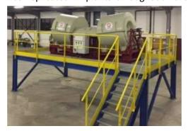
treat up to 10 tons/day and will include a Salter Cyclones SCMG2 Multi-Gravity Separator. Due to the wide variations of the feed material, the SCMG2 supplied can operate within a wide range of slope angles, shake speed, amplitude and drum speed.
